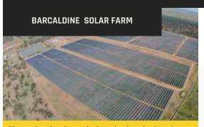
The project has been designed using single-axis tracking technology maximising the total energy generated and the effectiveness and efficiency of each of the panels.
